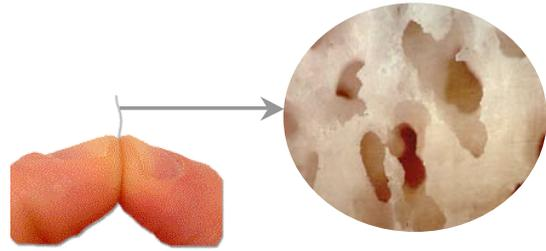
400x photo showing micropore structure of a SINGLE FIBRE from an AquaMat®. Each AquaMat® has millions.
